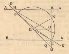
Let A a, B b be the planes which terminate the medium, and G H be the direction of the body's incidence, and I R that of its emergence.
